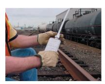
3. Holding in an upright manner, screw the mixing tube onto the top end of canister set. Make sure the mix tube assembly is secure.
