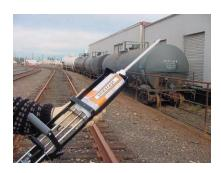
4. Place canister set into dispensing gun. Make sure the plunger assembly rods are level with the bottom of the canister set configuration, and that the nut is outside the frame.
