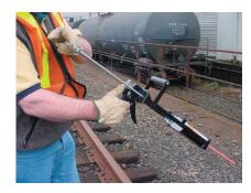
9. To remove empty canister, depress and hold lever on the back of the trigger and pull plunger rod back to start position. Pull canister out and discard.
