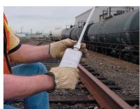
3. Holding in an upright manner, screw the mixing tube onto the top end of canister set. Make sure the mix tube assembly is fully secured.
