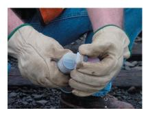
2. Remove the black plug caps from the canister set, while holding canister upright.
