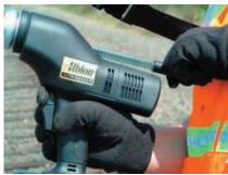
9. To remove empty canister, depress top portion of the trigger and pull plunger rod back to start position. Pull canister out and discard.
