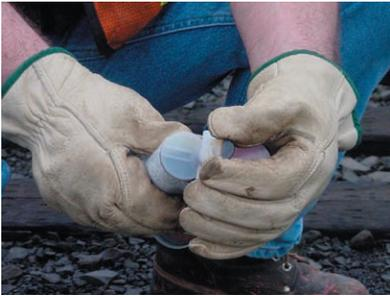
2. Remove the black plug caps from the canister set, while holding canister upright.
