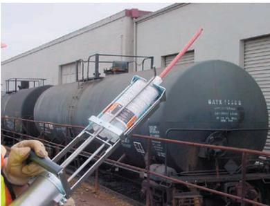
5. Hold dispensing gun upright and depress the bottom portion of the trigger until plunger rods make contact with canister.
