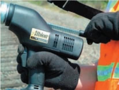
9. To remove empty canister, depress top portion of the trigger and pull plunger rod back to start position. Pull canister out and discard.
